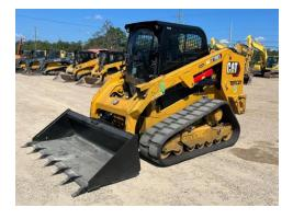
• **Condition**: GP bucket in good shape with no cracks, excessive wear, or missing teeth. Edges inspected and found within wear limits.
